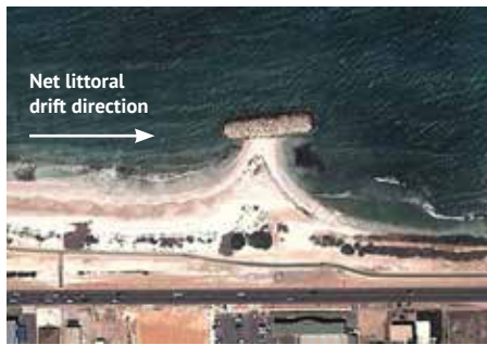
Photo 5 and Photo 6: Beach Tombolo created in lee of an offshore breakwater in Geraldton, Western Australia (Credit: Shand)
